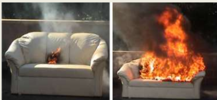
A previous example of unsafe burning furniture, at 1 minute and 2½ minutes respectively
